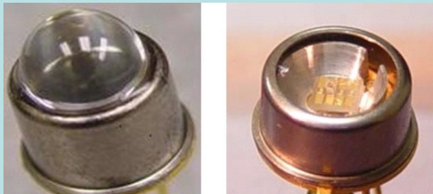
Deep – UV LEDs \lambda \approx 260 nm
