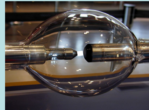
15 kW Xenon arc lamp
