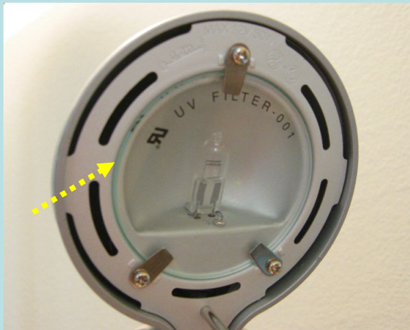
A Tungsten-Halogen lamp with a filter (arrow) to remove UV light.
